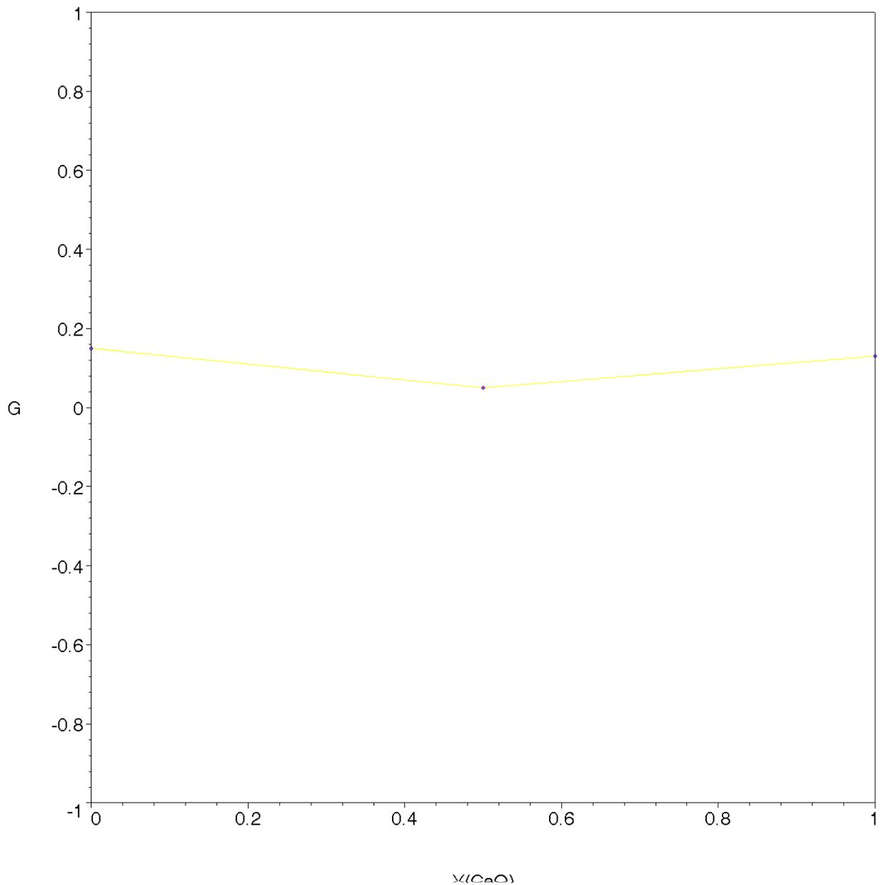
by raising the temperature to 26, the gm-x coordinate of wollastonite ( $x=0.5$ ) can be made to move off the minimum free energy surface of the system.
