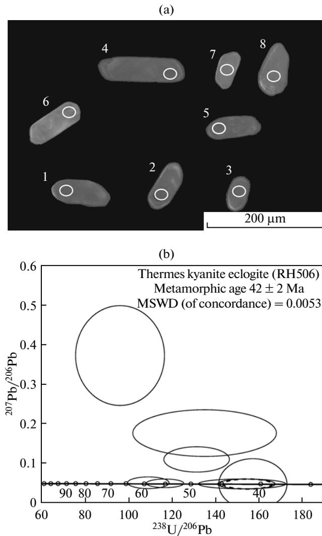
**Fig. 6.** (a) Cathodoluminescence (CL) image of zircon grains separated from the Thermes kyanite eclogite. (b) Tera-Wasserburg diagram for measured zircons from the Thermes kyanite eclogite and calculated concordia age of  $42 \pm 2$  Ma, ( $2\sigma$ , decay-constant errors included, probability of concordance 0.94). Two zircon dates yield a concordant age of around 55–60 Ma.
