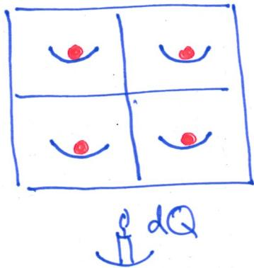
$\rightarrow dS = dQ/T \rightarrow$  reversible limit, all heat converted to vibrational entropy.
