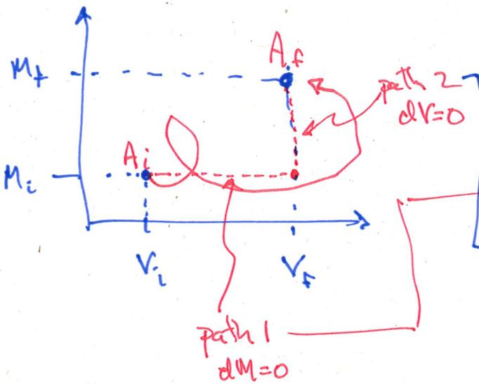
$$\Delta A = \int_{V_i, M_i}^{V_f, M_f} dA = \int_{V_i, M_i}^{V_f, M_f} (-P)dV + \int_{V_i, M_i}^{V_f, M_f} \mu dM$$
